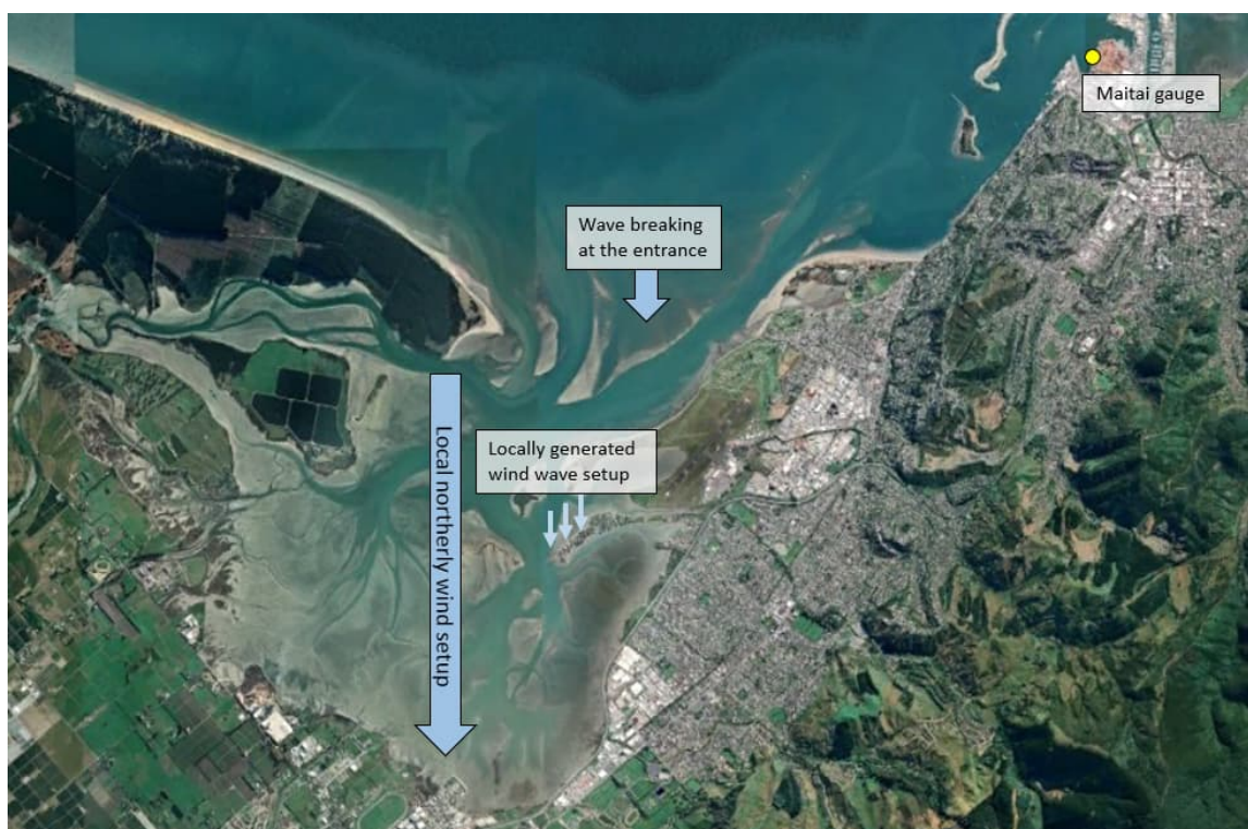
Figure 3.4: Schematic showing the potential setup components contributing to different levels in the Waimea Inlet.
