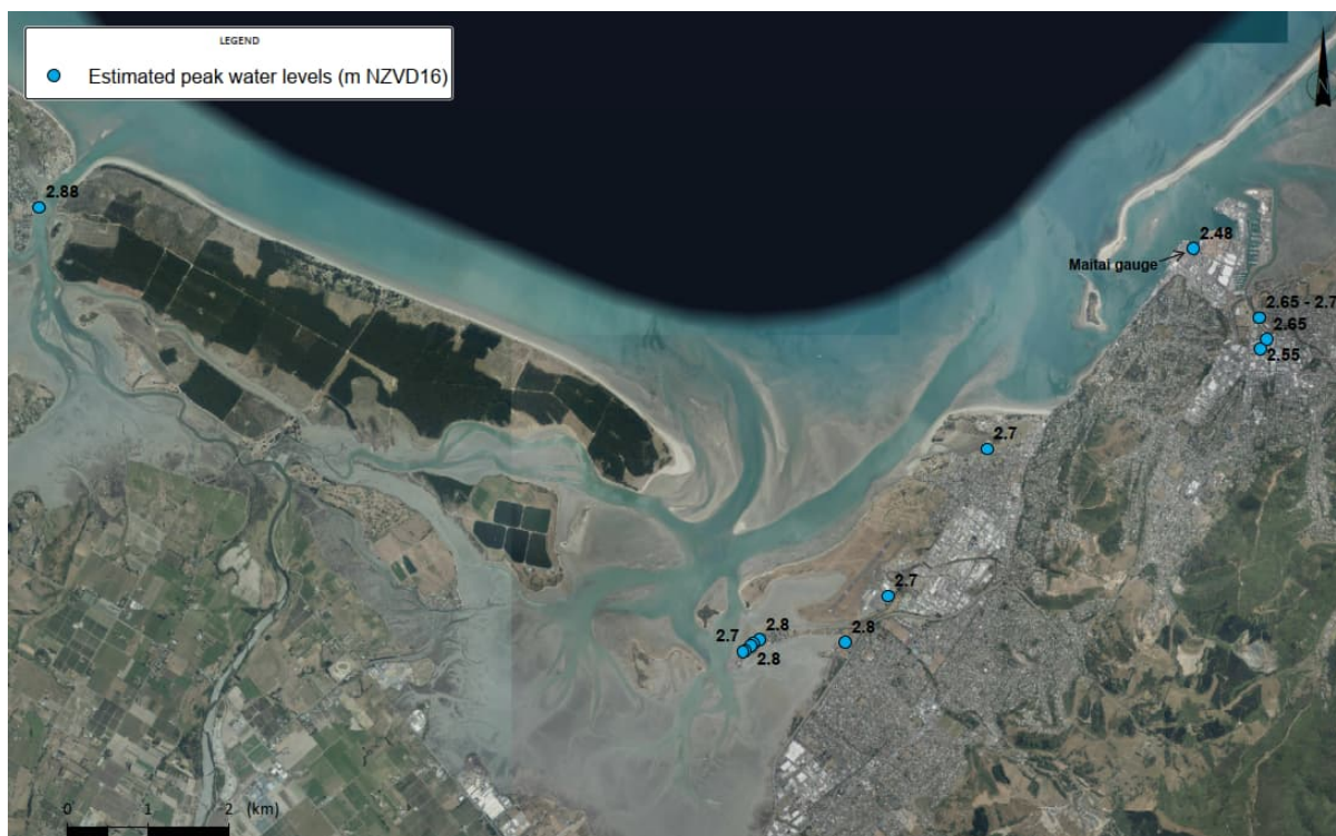
Figure 3.3: Estimated peak water levels based on observations and photos taken during Ex TC Fehi
