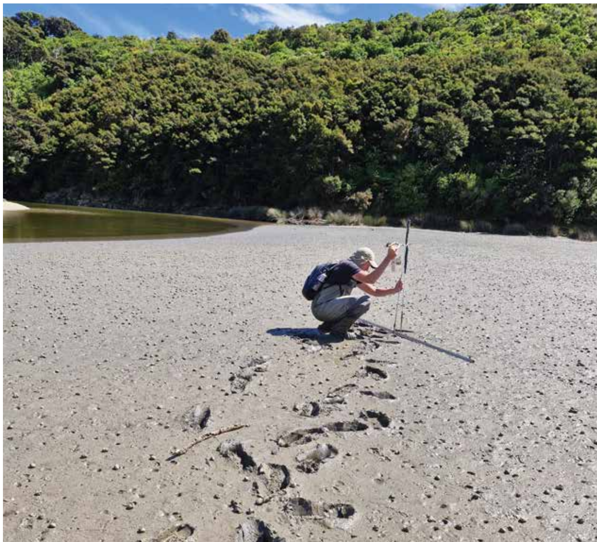
Picture 27: Measuring Sediment Plates in Kokorua Estuary. Photo credit P. Fisher
